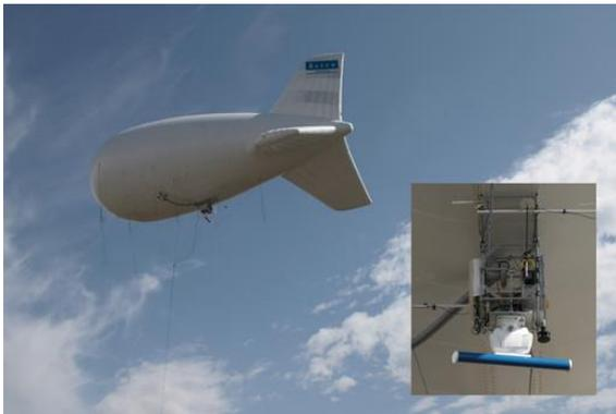
**Aerostats.** The aerostat is a fixed site, tethered airborne sensor platform. Many configurations are available. The U.S. armed forces have deployed them extensively in Iraq and Afghanistan to provide perimeter security surveillance for remote bases of operation in support of coalition forces. The same systems can provide outstanding support for security surveillance of any perimeter, along borders, high value assets, etc. Depending upon
